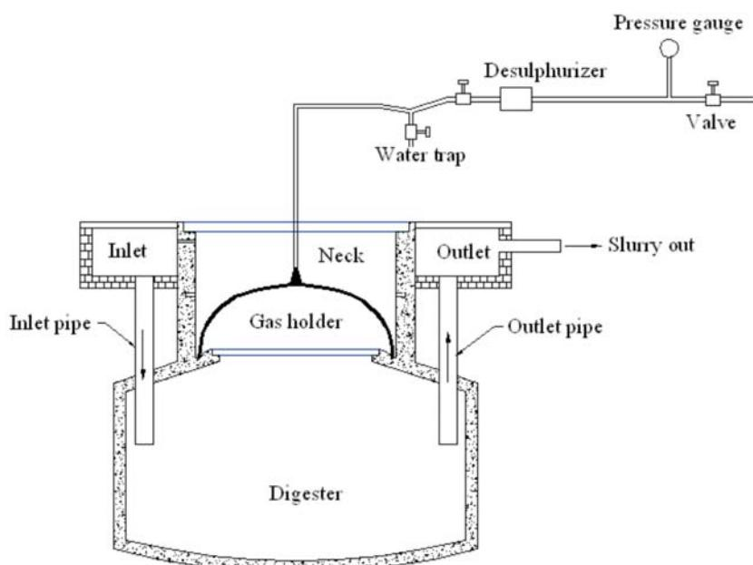
Figure 6.2: Schematic diagram of Puxin model biogas plant
