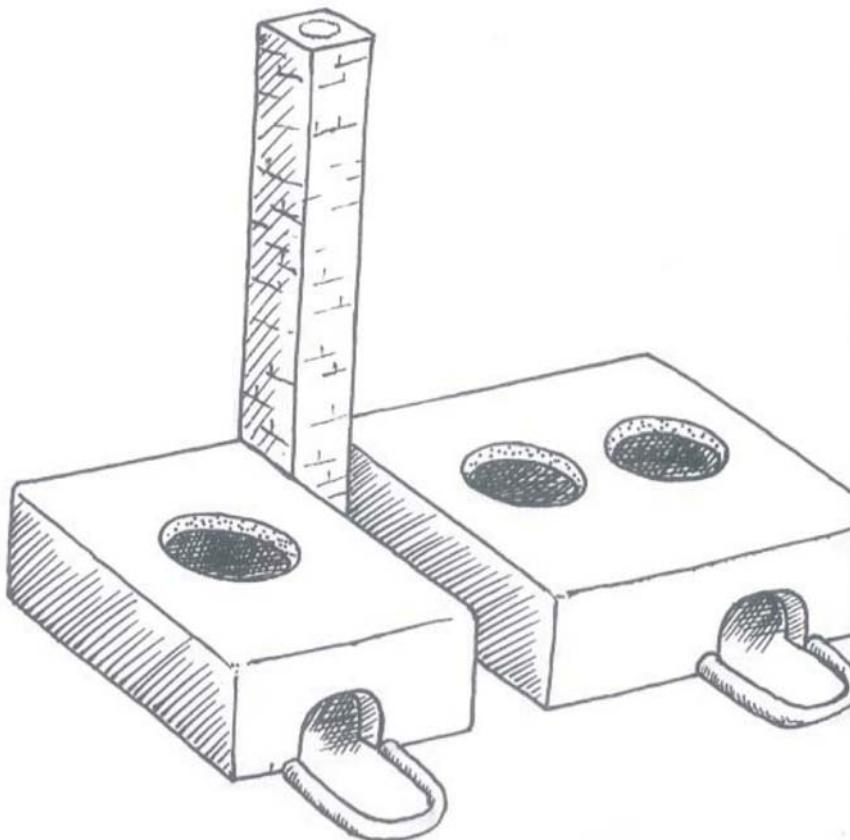
Figure 3.11: Three potholes multipurpose ICS
