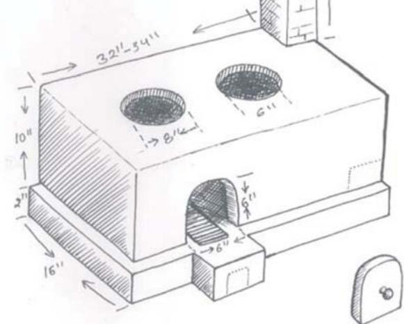
Figure 3.5 Two potholes ICS with raised second pothole
