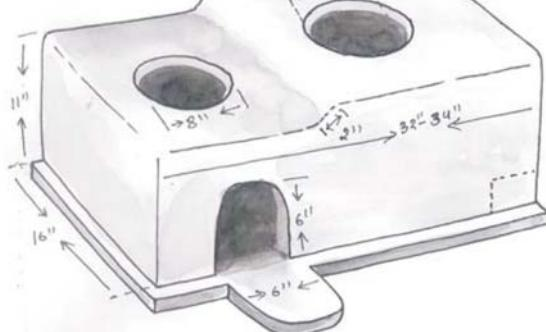
Figure 3.6 Two potholes ICS with grate
