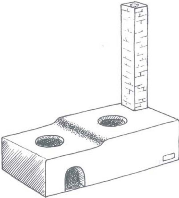
Figure 3.10: The second pothole raised two potholes ICS at waist height
