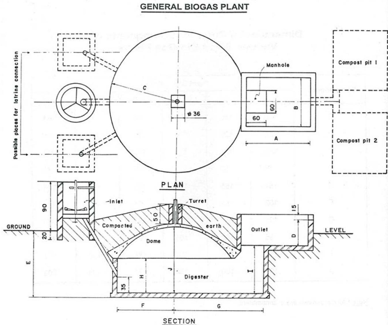
Figure 6.1: GGC 2047 model biogas plant
