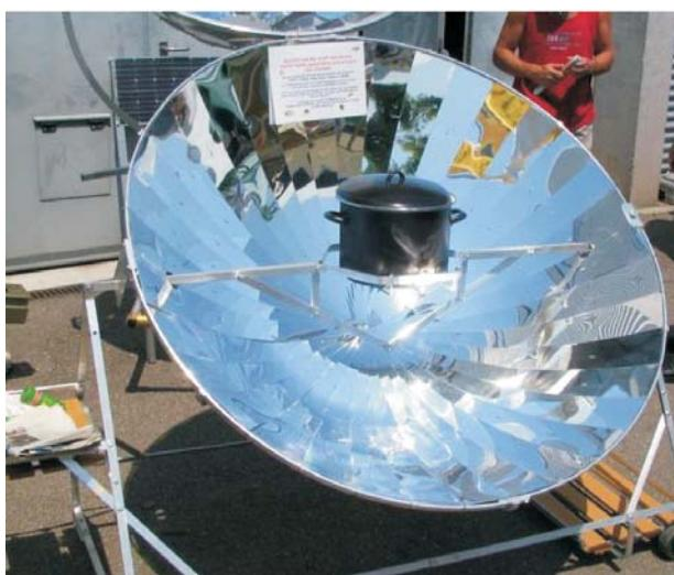
Parabolic type solar cooker
