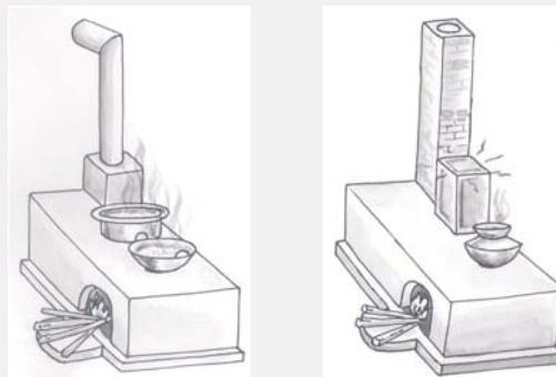
Figure 3.8: Metal chimney and use of tin for space heating
