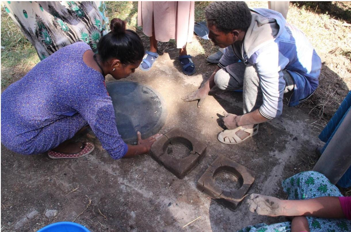
The chimney-bricks are air-dried, not fired
