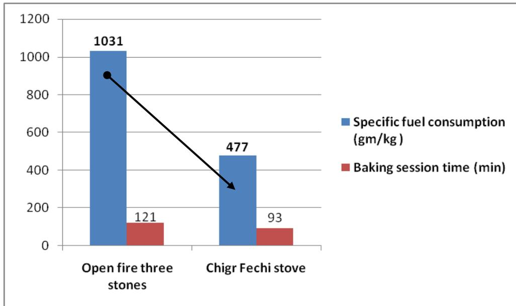
**Figure 5: Performance of Chigr Fechi Injera baking as compared to open fire stove**
